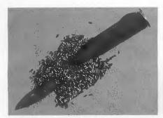
Outwardly this round of 7N1 simply looks like an ordinary ball round manufactured at Factory 188 in 1981. However, pulling it apart reveals a longer projectile with a hollow base.
